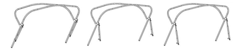
To release the adjustable struts for stowing the top simply pull down slightly on the leading edge of the top and press the locking lever to release the tension on the top. Repeat on both sides. With the bimini now relaxed you can unfasten the adjustable struts from the mounting buttons, fold the bimini towards the back of the boat and put on the storage boot.
